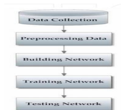
Figure-5: Basic flow for designing artificial neural network model
